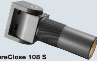
SureClose 108SF S Code: 75108123m SELF-CLOSING FROM 90° • With final snap-close action • Gate sweep: 90° in and out • No hold-open feature (suitable for pool/safety gates) • Adjustment tool included
